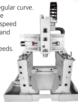
• High vibration damping capacity of cast iron base.
